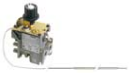
VÁLVULA EUROSIT 110÷190°C BURNER BASE, 5.5KW Cod. EMMEPI: 808934 Cod. IBERITAL: 40499
